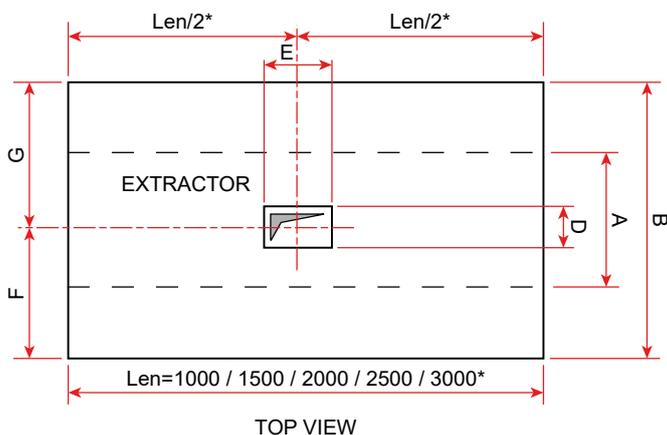
\* Hood length 3000 mm composed as standard of a 2000 + 1000 mm module (3000 mm single block as an option)
